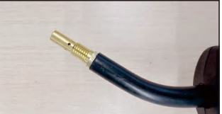
Insert the new liner into the gun from the back end, pushing it all the way through until it exits at the front end.
