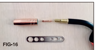
Install the matched aluminum A+ contact tip and nozzle back into the MIG gun.
