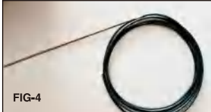
Take out the graphene liner (black).
