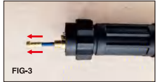
Pull out and completely remove the liner.
