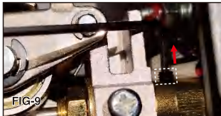
Use a small hex wrench to unscrew the black hex screw on the outlet guide tube.
