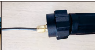
Install the liner retainer and nut onto the back end of the gun.
