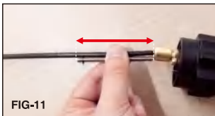
Cut a same length of liner as the outlet guide tube with wire cutter.
