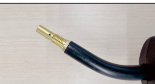
Insert the new liner into the gun from the back end, pushing it all the way through until it exits at the front end.
