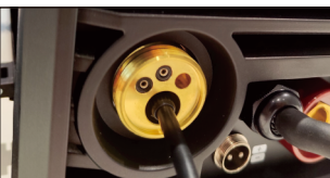
Remove the drive roller cap and drive roller.
