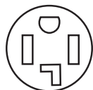
4-wire receptacle 14-30R
