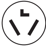
3-wire receptacle (10-30R)
