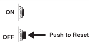
Receptacle Circuit Breakers
