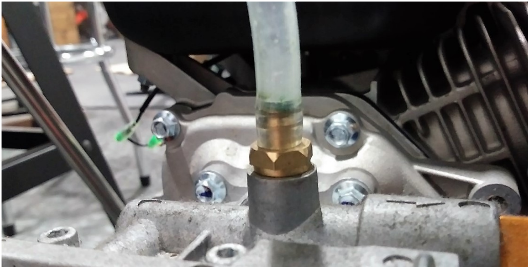
Fig. 3: Remove hose from fitting.
