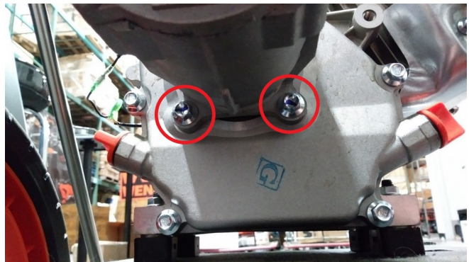
Fig. 5: Bottom pump-mounting screws.
