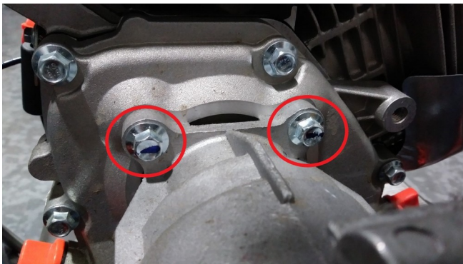
Fig. 4: Top pump-mounting screws.
