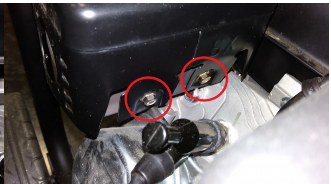
Fig. 2: Remove these 2 screws.
