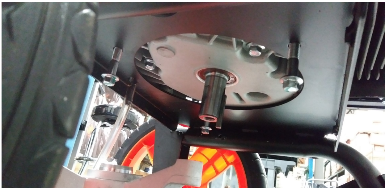
Fig. 8: Screws helping to align the engine on the frame.
