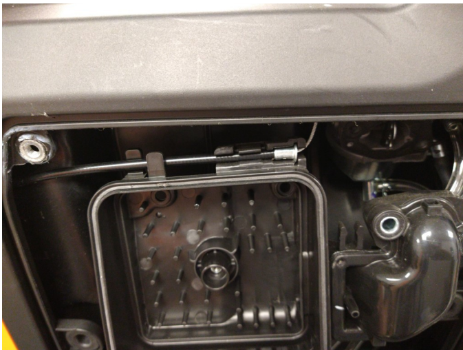
Fig. 8: Choke cable anchored in air filter housing.
