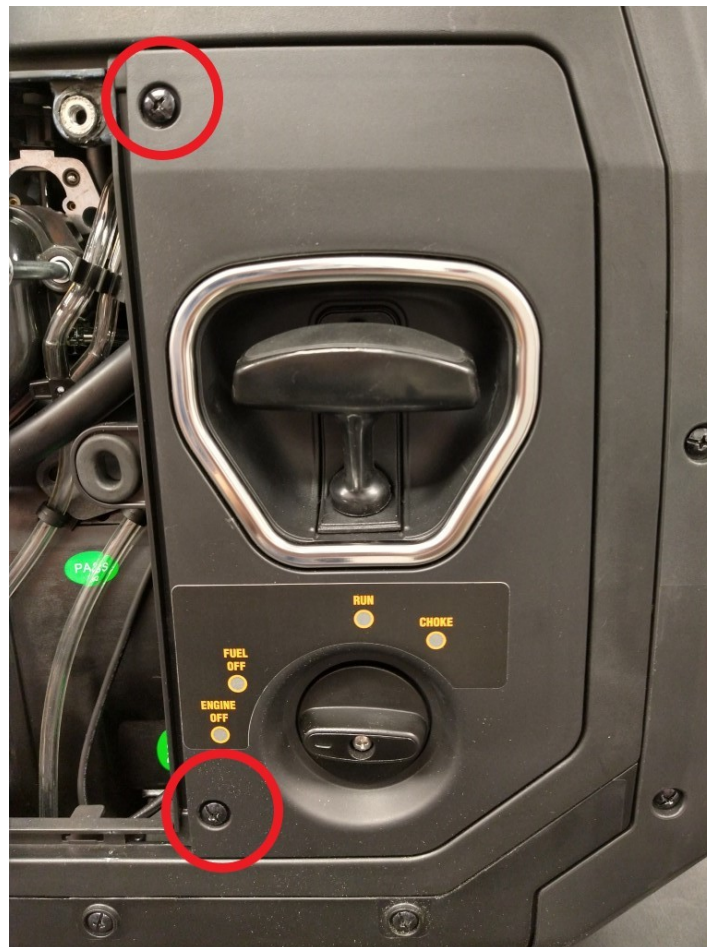
Fig. 3: Remove the two Phillips-head screws, then pull the panel out.
