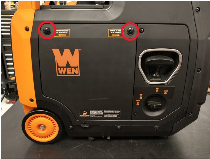
Fig. 1: Remove the screws, then the panel.
