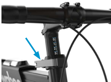
Stack Height Adjustment
