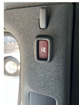
Figure 10-6: Sliding Door Switch
