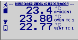
Device type and user defined Device ID are displayed on the Home Screen.
