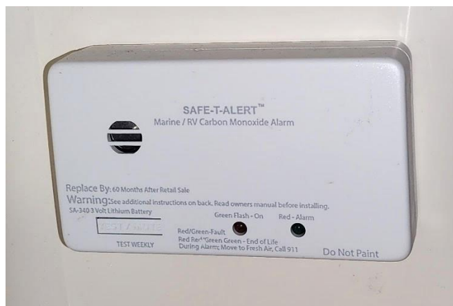
CO Detector & Alarm
