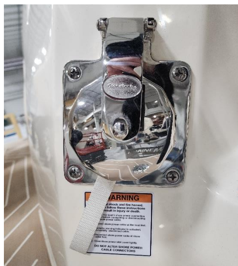
Shore Power Inlet Cover
