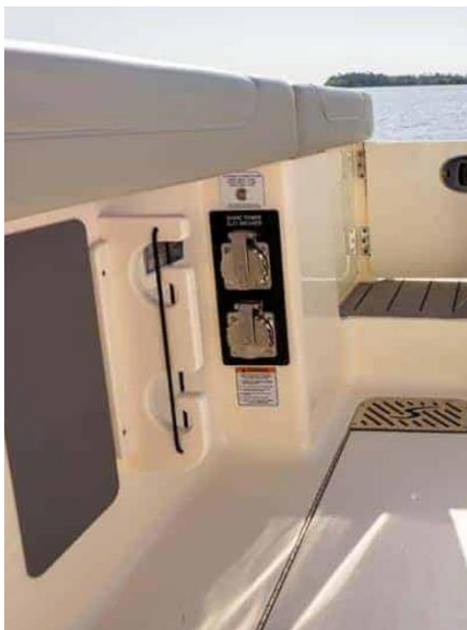
Starboard Shore Power Panel
