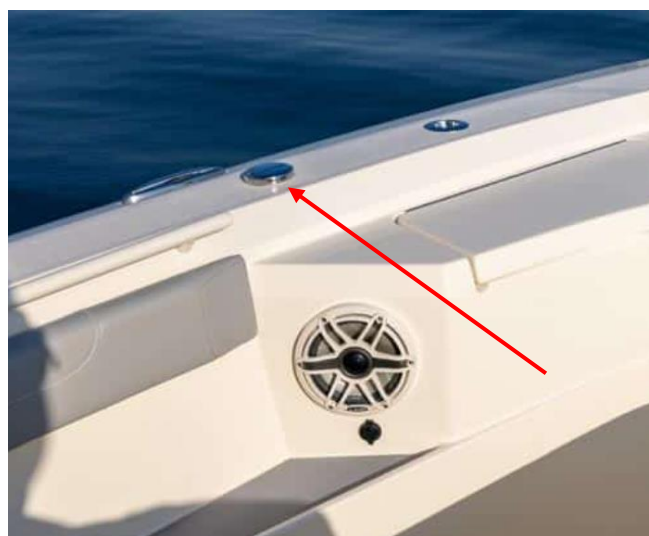
Fresh Water Fill
