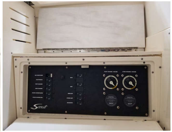
Battery Switch Panel Underneath Console Step
