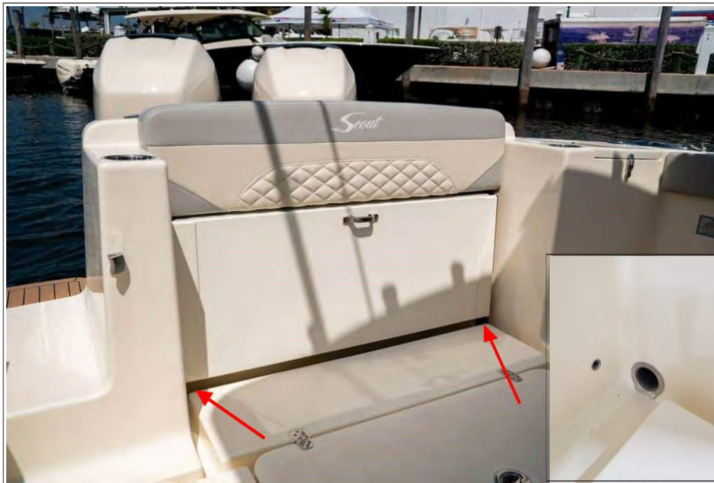
Port & Starboard Cockpit Scupper Drains
