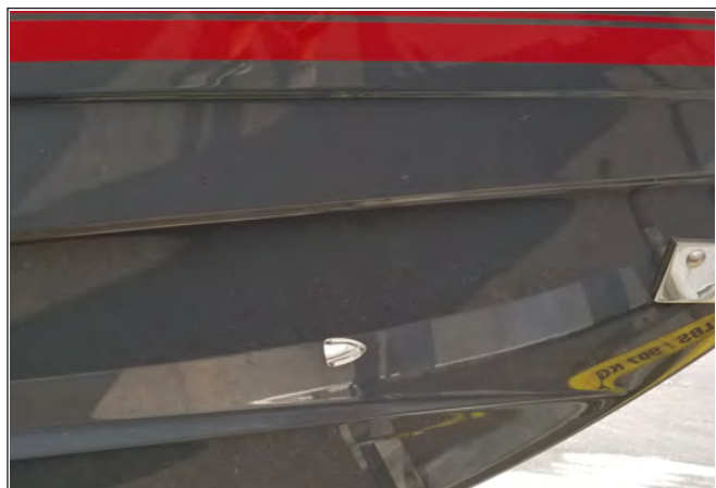
Typical Rope Locker Drain
