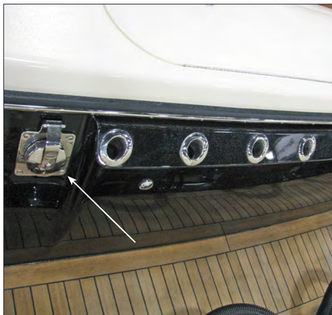
Shore Power Inlet Cord Hawse Pipe
