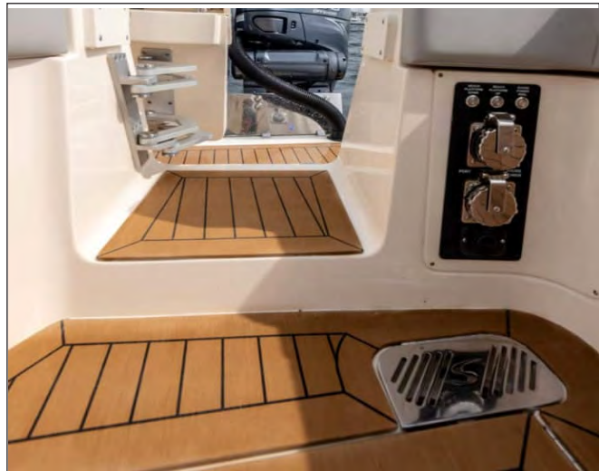
Beach Platform & Shore Power Reel Switches
