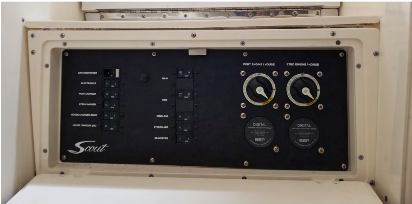
Dual Engine Battery Switch Panel, Motorized Battery Switches, Remote Battery Switches, Parallel Switches & Circuit Breakers
