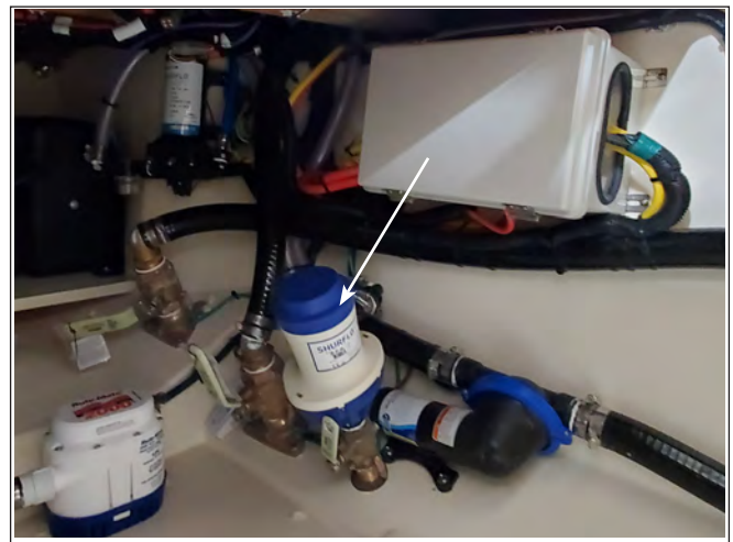
Baitwell Pump & Supply Valve Fitting
