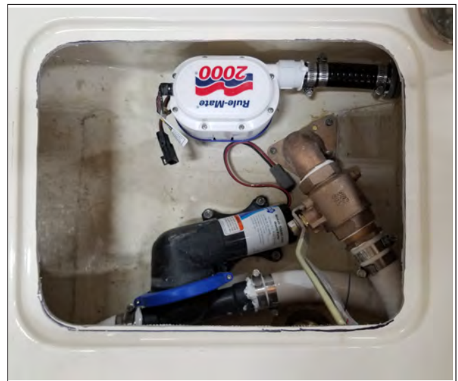
Forward Bilge Pump With Automatic Switch
