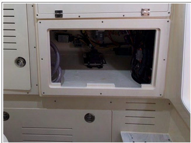
Helm Access Panel In Console
