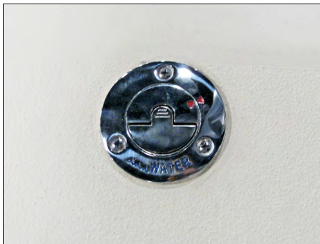
Fresh Water Tank Deck Fill Plate
