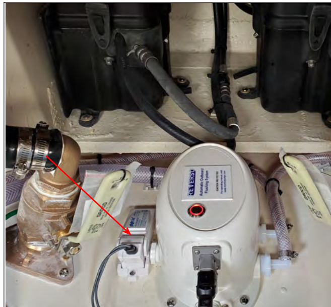
High Water Alarm Automatic Float Switch
