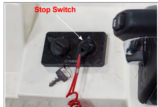
Yamaha Dual Engine Stop Switch All Engine Ignition START/STOP Switches
