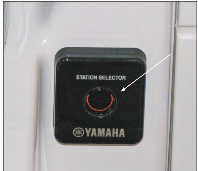
Typical Yamaha Triple Engine Station Transfer Button
