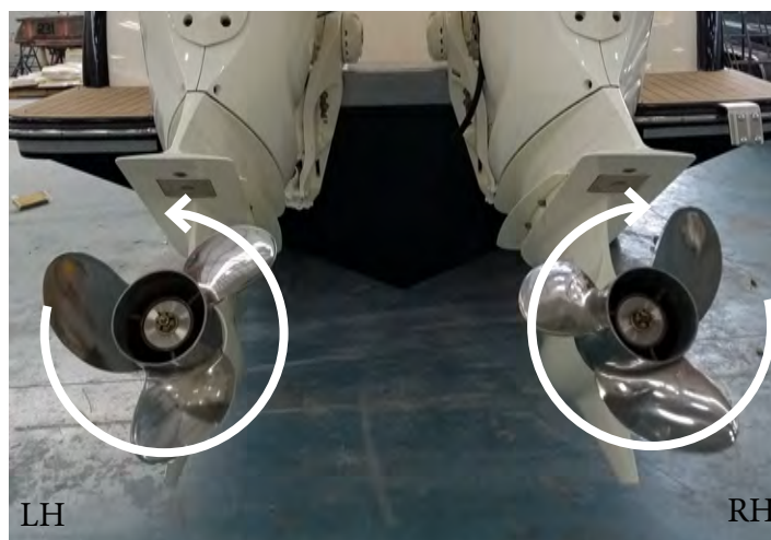
Typical Dual Yamaha Engine & Propeller Rotation
