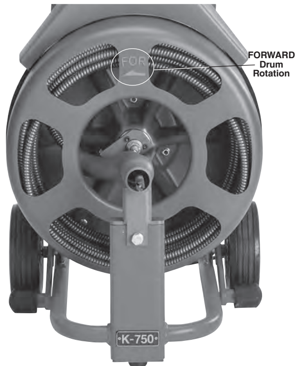
Figure 6 – Proper Drum Rotation (FOR Switch Position)
