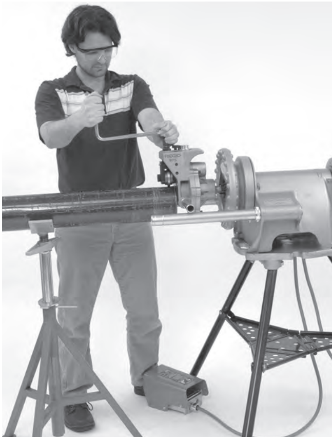
Figure 12 – Position de rainurage appropriée
