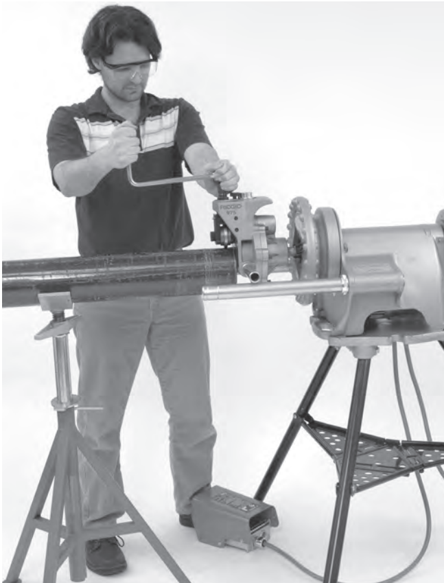
Figure 12 – Roll Groover Operating Position
