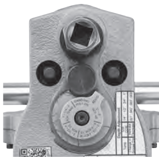
Figure 10B – Gauge In Grooving Position
