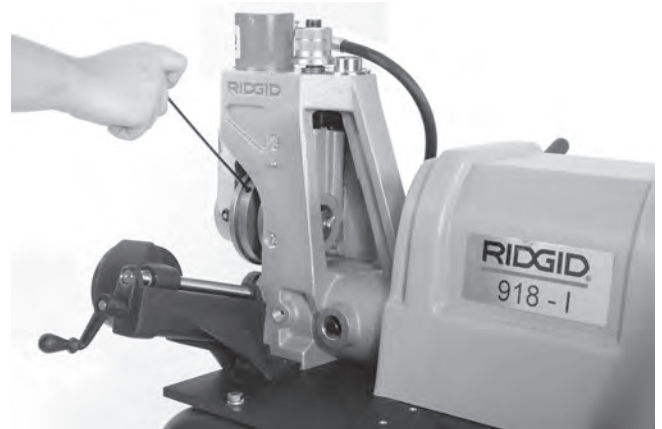
Figure 21 – Loosening Grooving Roll Set Screw
