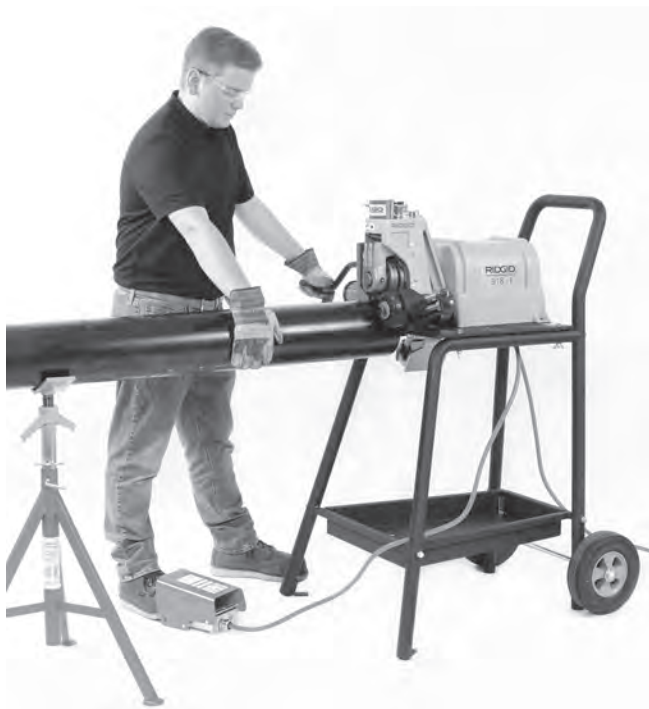
Figure 17 – Applying Pressure on Pipe
