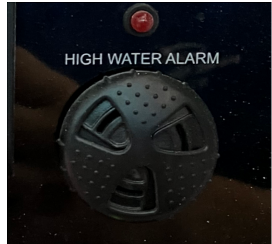
High water alarm
