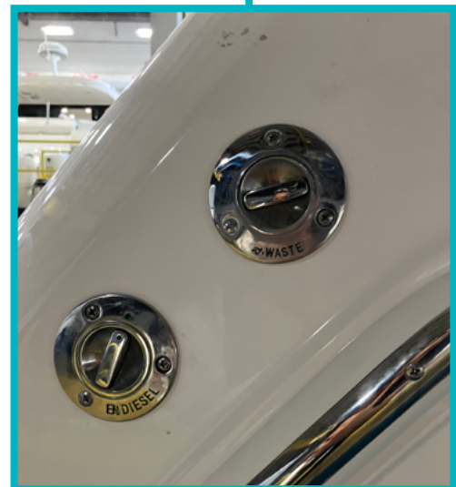
Diesel fill fitting and waste pump-out
