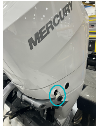
Mercury flush location
