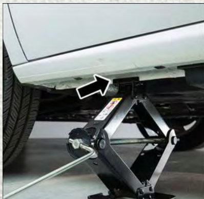
Front Jacking Location Engaged
