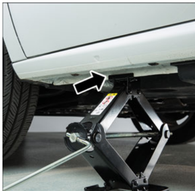
Front Jacking Location Engaged
