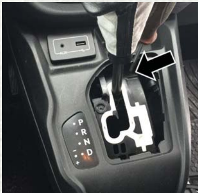
Gear Selector Override Access Hole
