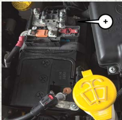
Positive Battery Posts
