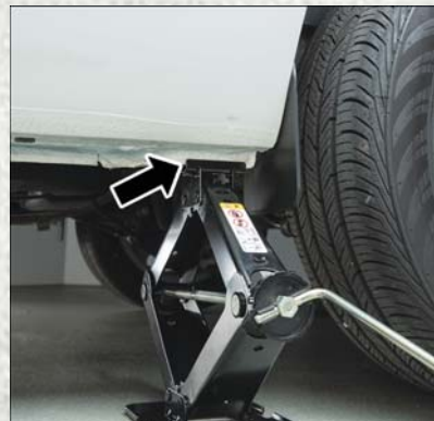
Rear Jacking Location Engaged
