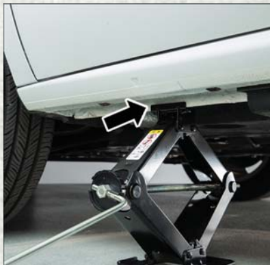
Front Jacking Location Engaged
