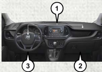
Front Air Bag/Knee Impact Bolster Locations
