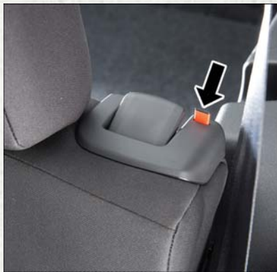
Seatback Latch Indicator Unlocked Position
