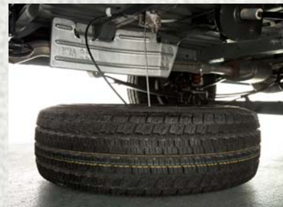
Lowering Spare Tire
