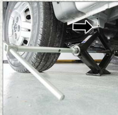
Front Jacking Location
