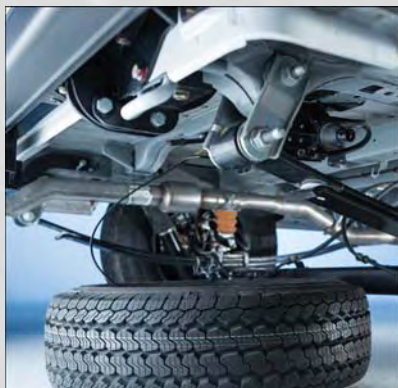
Lowering Spare Tire
