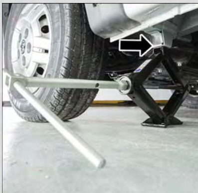
Front Jacking Location
