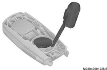
Key Fob Battery Removal
