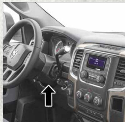
Gear Selector Override Access Port
