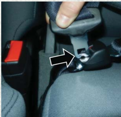
Detaching Mini-Buckle With Seat Belt Tongue
