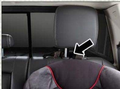
Tether Strap Through Outboard Tether Strap Loop
