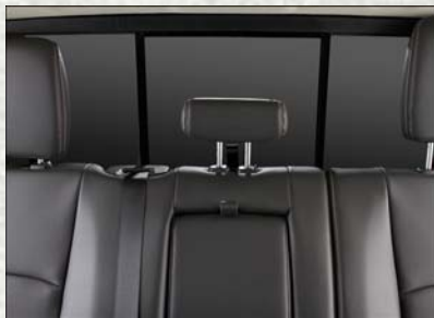
Tether Strap Loop With Center Head Restraint In Raised Position
