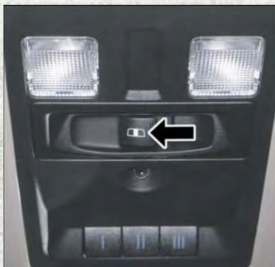
Power Sliding Rear Window Switch
