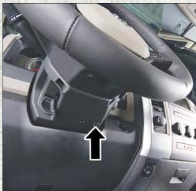
Shift Lock Manual Override Access Port
