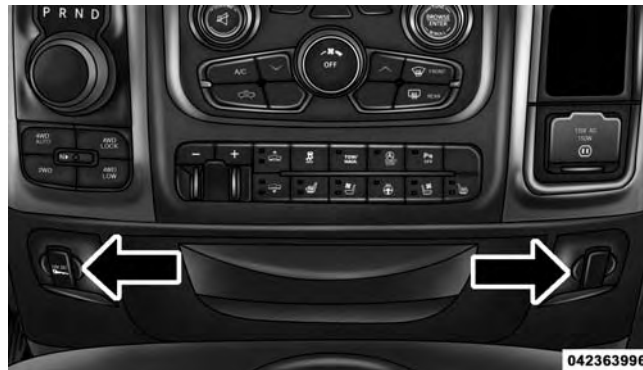
Power Outlets — Center Stack
