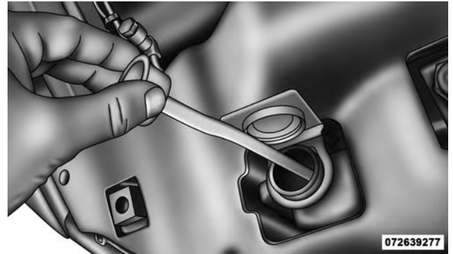
Coolant Reservoir Dipstick
