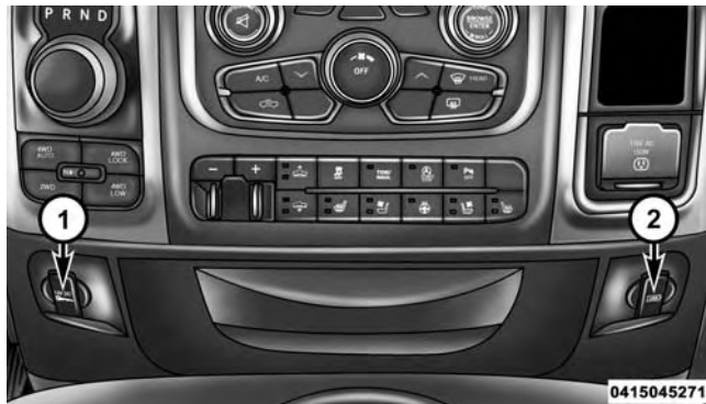
Power Outlets — Center Stack
