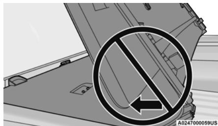
Incorrect Folding – Will Cause Damage
