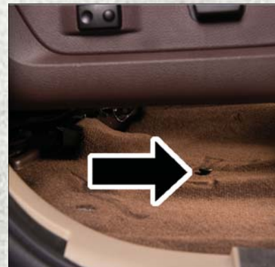
Floor Fastener Location
