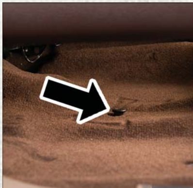
Floor Fastener Location
