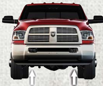
Front Jacking Location
