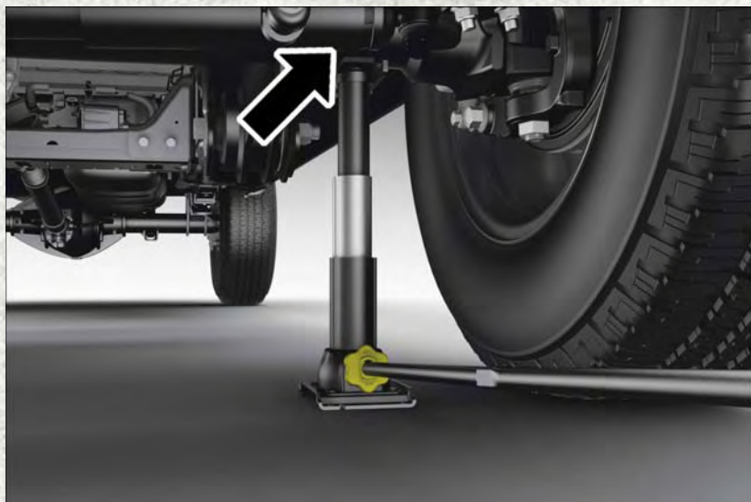
Front 4x2 Jacking Location
