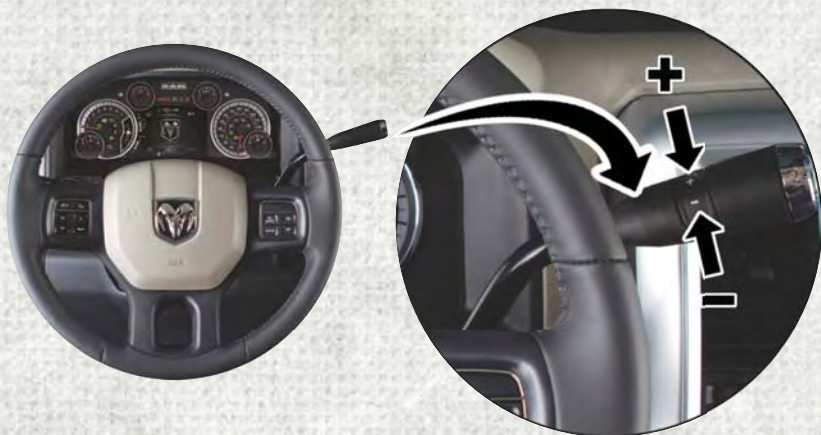
ERS Control On The Gear Selector
