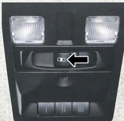
Power Sliding Rear Window Switch
