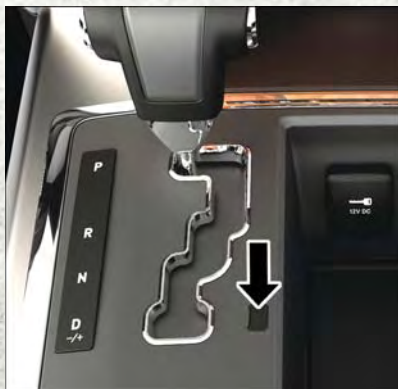
Gear Selector Override Access Cover
