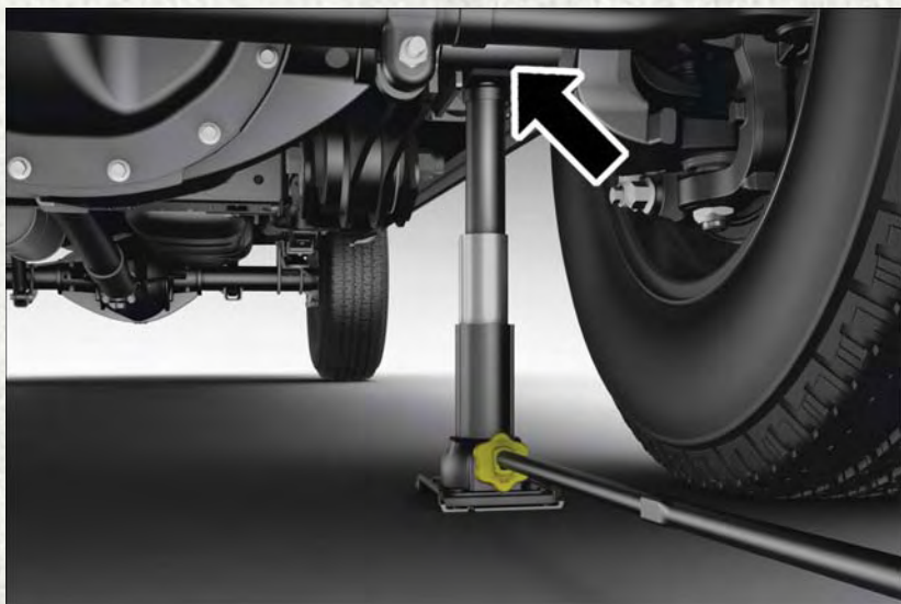
Front 4x4 Jacking Location
