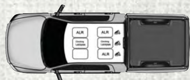
Quad Cab/Mega Cab/Crew Cab Automatic Locking Retractor (ALR) Locations
