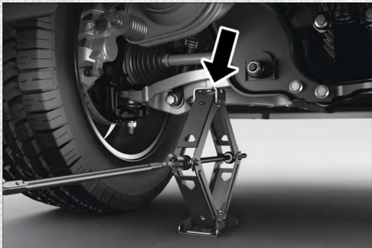
Front 4x4 Jacking Location
