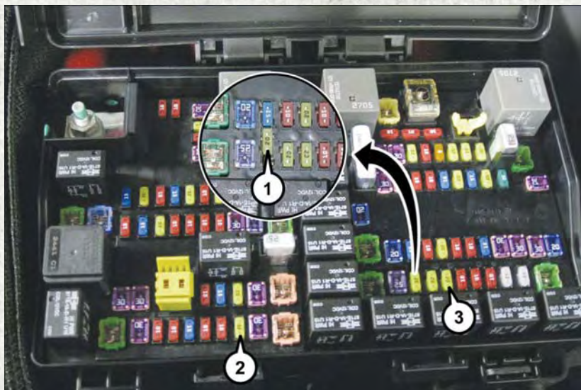
Power Outlet Fuse Locations
