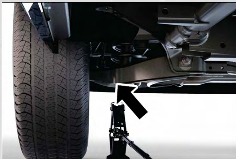
Front 4x2 Jacking Location
