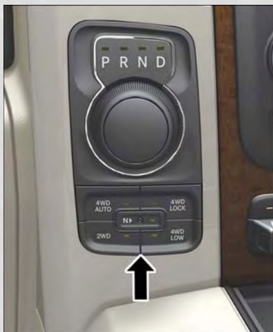
Five-Position/On-Demand Transfer Case — Eight Speed Transmission Only
