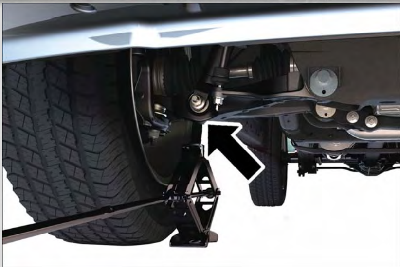
Front 4x4 Jacking Location
