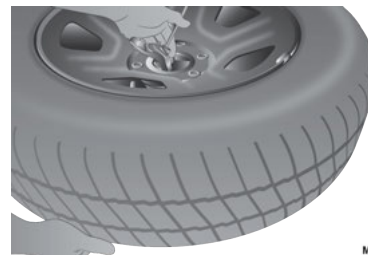
Pushing The Retainer Through The Center Of The Wheel And Positioning It
