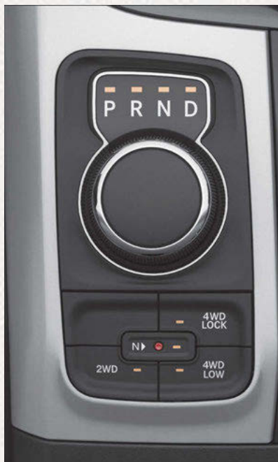
Four-Position/On-Demand Transfer Case — Eight Speed Transmission Only
