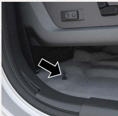
Floor Fastener Location
