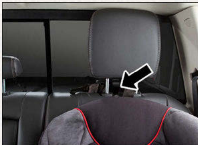
Tether Strap Through Outboard Tether Strap Loop
