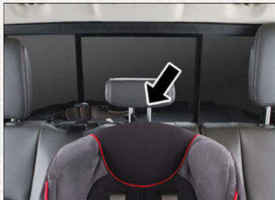
Tether Strap Through Center Tether Strap Loop
