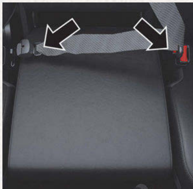
Mini-Latch And Mini-Buckle Connected
