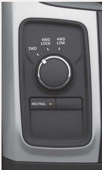
Four-Position/Part Time Transfer Case
