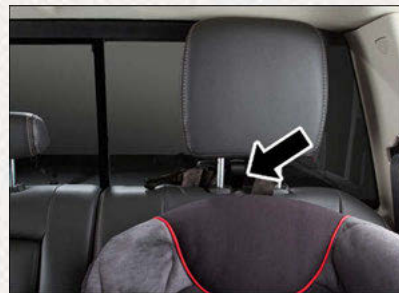
Crew Or Quad Cab Outboard Tether Anchorage
