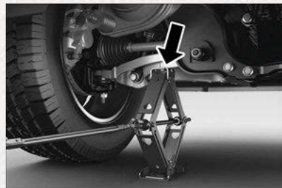
Front 4x4 Jacking Location
