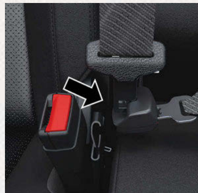
Detaching Mini-Buckle With Seat Belt Tongue
