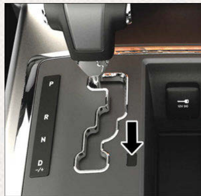
Gear Selector Override Access Cover
