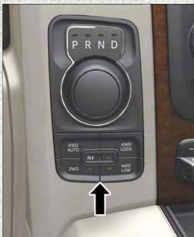
Five-Position/On-Demand Transfer Case — Eight Speed Transmission Only
