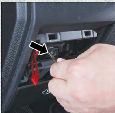
Manual Park Release Lever Locking Tab
