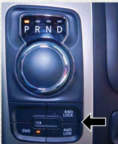
Four-Position/On-Demand Transfer Case — Eight Speed Transmission Only
