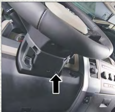
Shift Lock Manual Override Access Port
