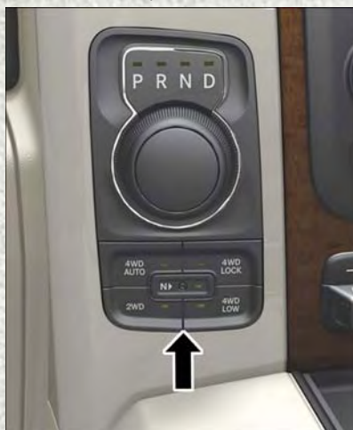
Five-Position/On-Demand Transfer Case — Eight Speed Transmission Only
