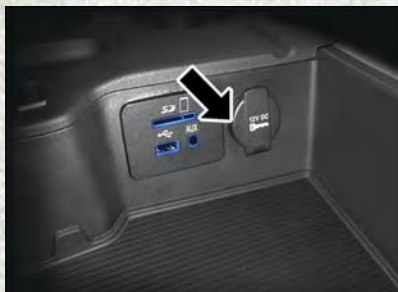
Power Outlet — Storage Compartment
