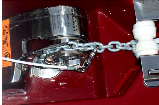
Anchor Chain Secured
