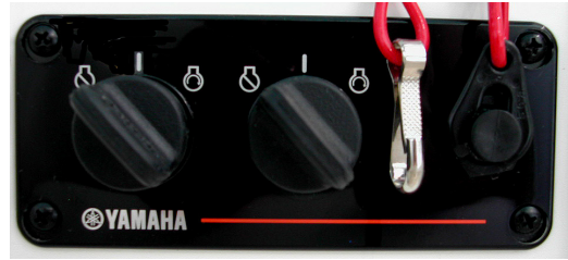
Engine Stop Switch
