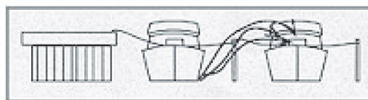
NEARBY BOAT GENERATOR EXHAUST
