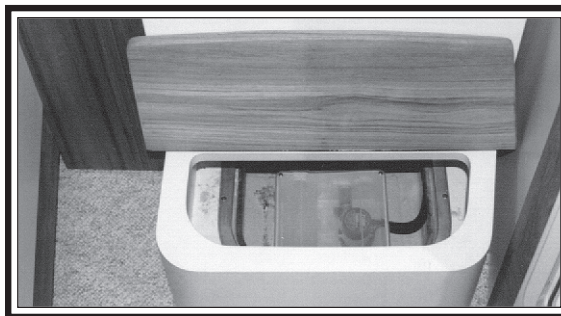
Shower and Cabin Drain Sump Pump
