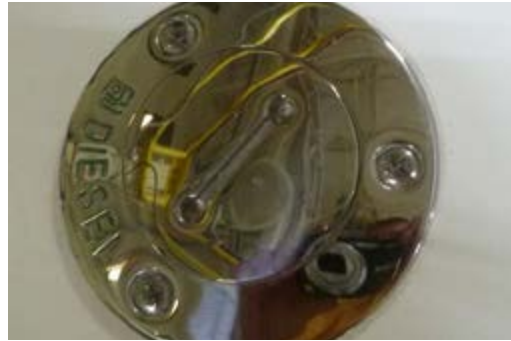
Diesel fuel fill
