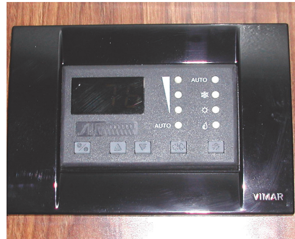
Air Conditioning Control Panel
