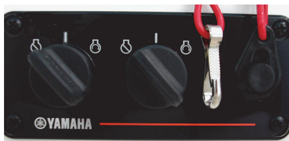
Engine Stop Switch Lanyard (Typical)
