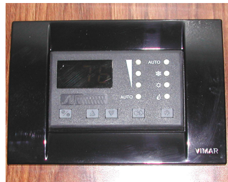
Air Conditioning Control Panel
