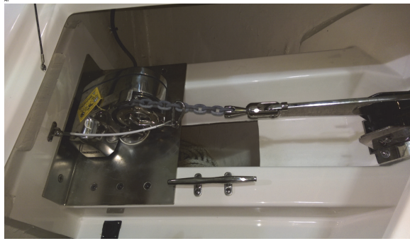
Anchor Line Secured Using Cable
