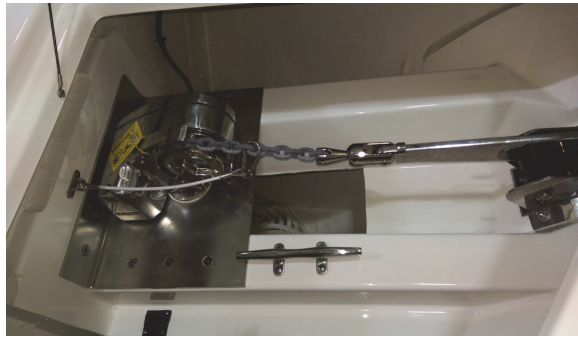
Anchor Line Secured Using Cable
