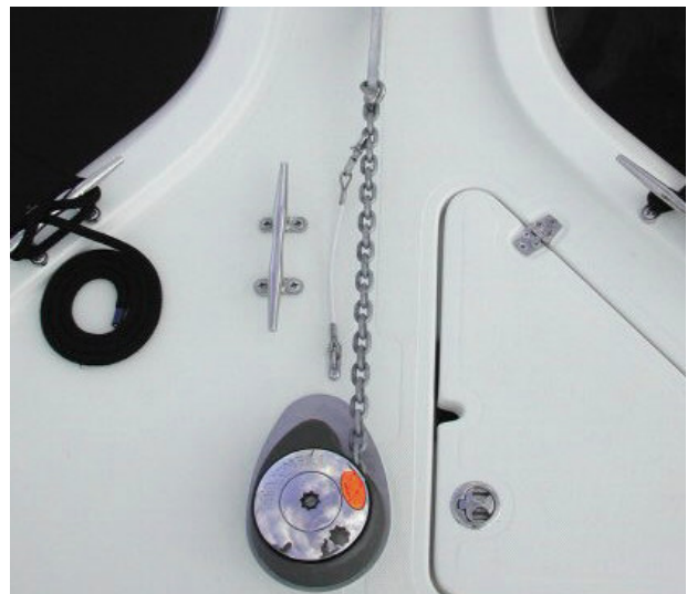
Anchor Chain Properly Secured For Travels
