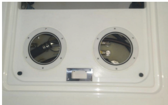
Gas Tank Valves
