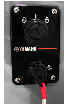
Engine Stop Switch
