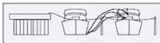
NEARBY BOAT GENERATOR EXHAUST
