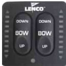
Trim Tab Switches
