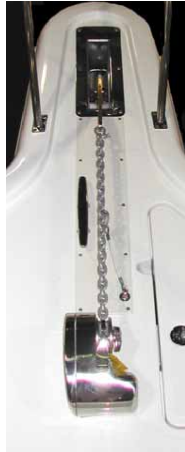
Anchor Chain Properly Secured for Travel
