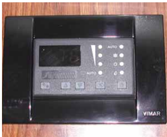
Air Conditioning Control Panel
