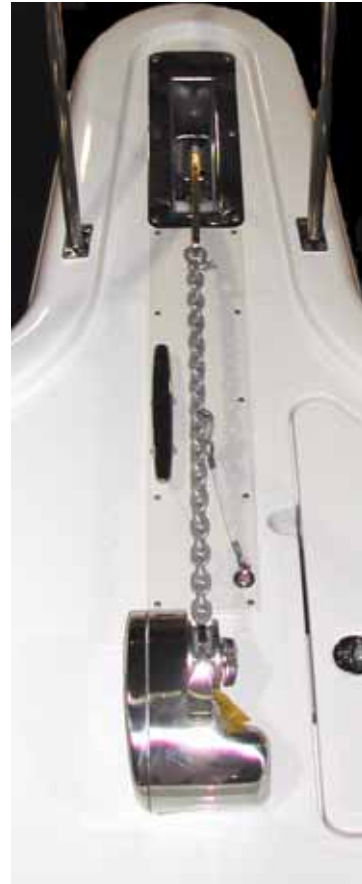
Anchor Chain Properly Secured for Travel
